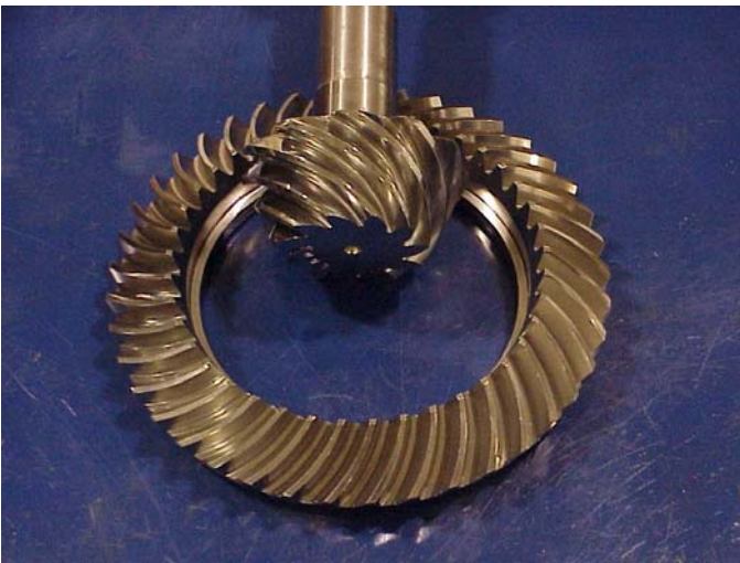
Figure 12. Gear set photo after superfinishing process
