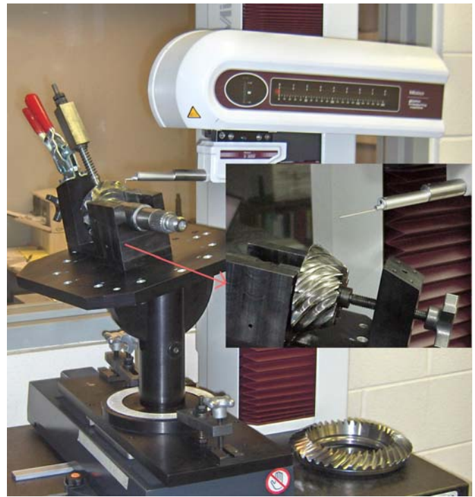
Figure 1. Form measuring machine setup
