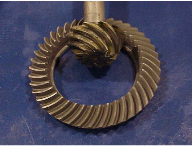
Figure 11. Gear set photo before superfinishing process
