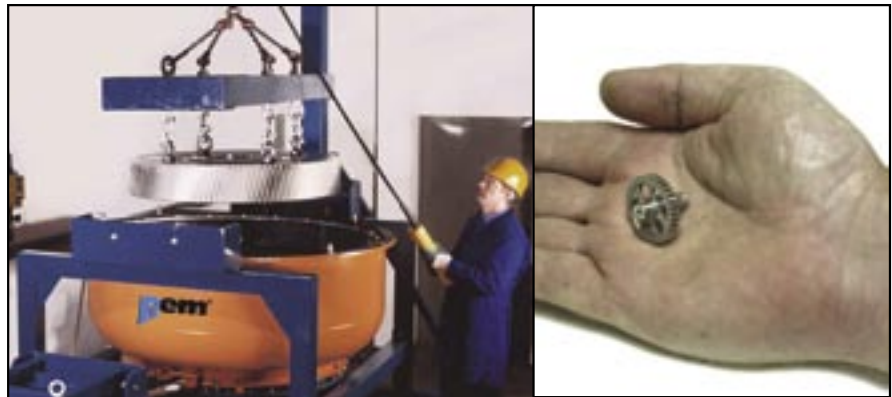
Before and After? No. —Gear manufacturers need not worry that superfinishing will have this effect on their gears. Skill is necessary in chemically accelerated vibratory finishing so gears retain their geometry, but it is a misconception that superfinishing distorts gear geometry.
