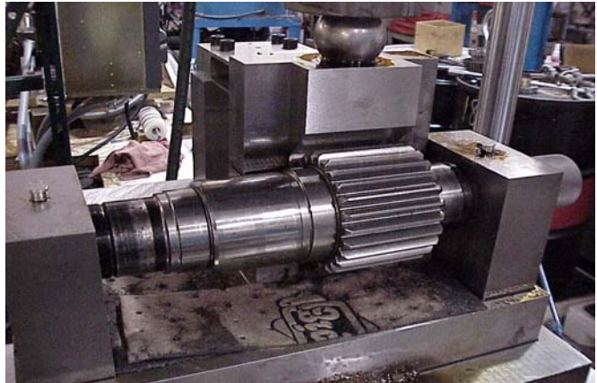
Figure 4. Single Tooth Fatigue Fixture
